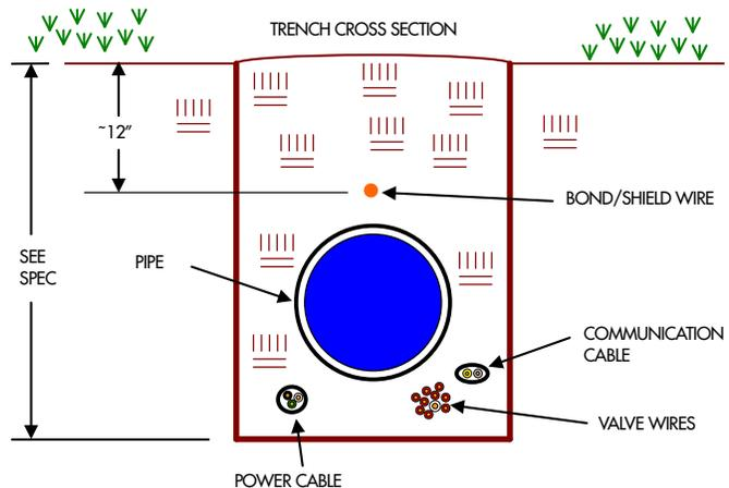
The conductor is laid in as straight a line as possible, and when necessary to make bends, do so in a sweeping motion as defined in the Installation section below. The shield network is to be connected to the service entrance earth ground, to all electronic equipment ground lugs, and all equipment supplementary grounding electrodes. One such network is necessary for each power source. **DO NOT INTERCONNECT THE EQUIPMENT GROUND WIRES FROM DIFFERENT POWER SOURCE SERVICE ENTRANCES.**
