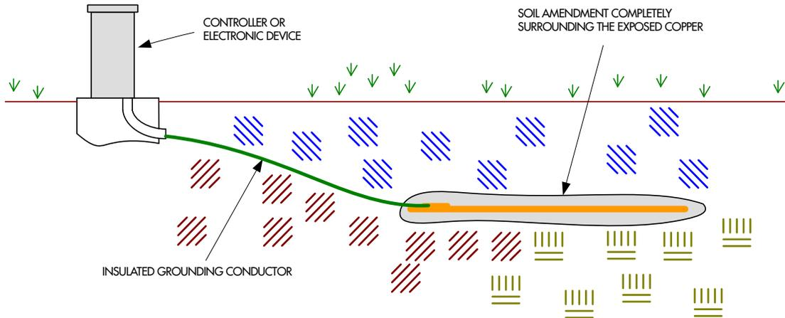
Install all grounding circuit components in straight lines and simple geometry. When necessary to bend wires, make sweeping turns as shown. All grounding and bonding wires of electronic equipment must be fed through a **dedicated 1.5” (38.1 mm) plastic sweep ell**. “Sweep bends” must follow the guidelines shown here.
