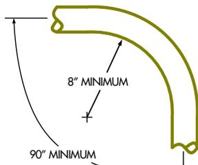
The 6 AWG bare copper wires are to be installed in as straight a line as possible, and if it is necessary to make a turn or a bend it shall be done in a sweeping curve with a minimum radius of 8” (203.2 mm) and a minimum included angle of 90°.
