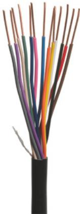
The irrigation cable shall incorporate enough wires to accommodate all the valves it is designed to control, plus some spares for future expansion. For example, if the cable will activate 6 valves, then the number of wires needed is: 6 hot + 1 common + 2 spares = 9 wires. This cable would be called out as 18 AWG/9c. The construction shall include insulated solid copper conductors and an overall PE jacket. The cable shall be listed as Underground Low Energy Circuit Cable.
