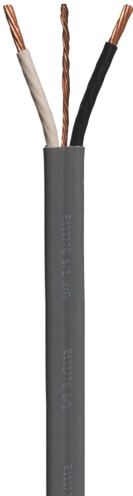
All branch circuit power cables shall be type UF-B. They are to be UL® listed for direct burial, and rated at 600 volts. The cable shall include “three conductors”. The inner copper conductors shall be insulated with high dielectric PVC and Nylon. The outer jacket will be gray PVC and is to be sunlight resistant. The inner conductors are colored black, white, and bare copper.
