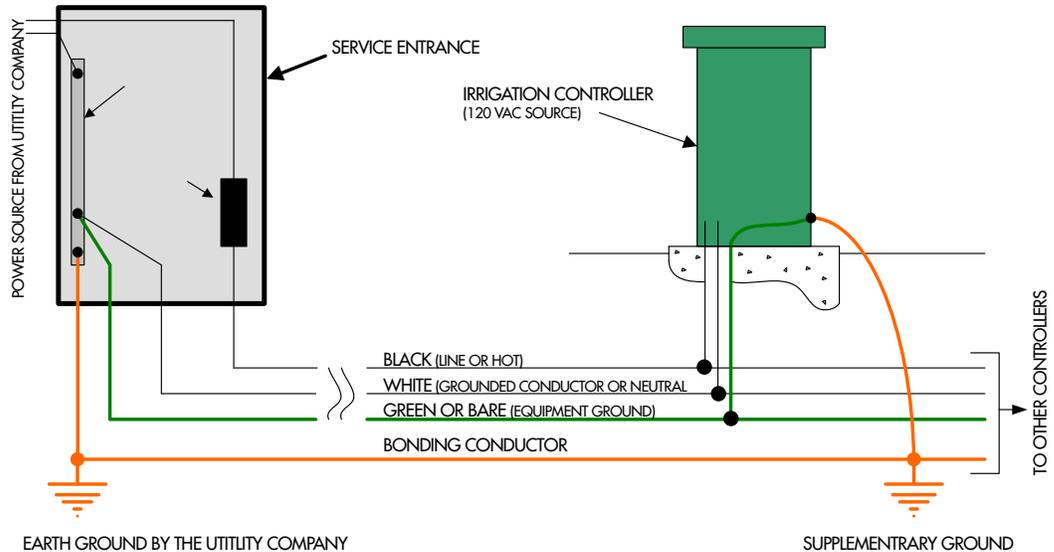
Vac power sources, the wires are Black, White and Green. For 240 Vac power sources, the wires are Black, Red and Green. Power wires must always be kept together in a trench, conduit, tray, etc. The bonding conductors are required to be 6 AWG solid bare copper, unless the system power conductors are larger than 1/0 AWG, in which case the bonding wires are to be 4 AWG solid bare copper.
